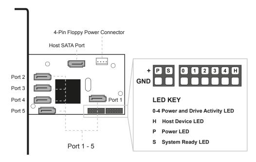
Note: When the internal port multiplier (PM) is connected to a SATA Host controller with Sil3124 or Sil3132 chip, in the RAID BIOS of the host controller, you will only see one drive and that is the drive connected to port 1 on the hardware PM.
